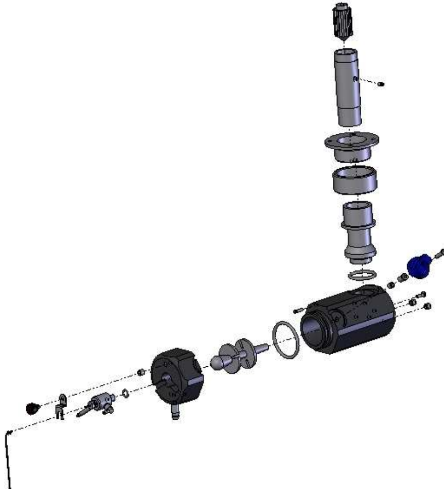
Figure 6.14 MK1 Mixing Chamber, Nebuliser and Burner assembly exploded diagram.
